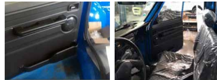
Design and Manufacturing of Nissan Pick Up Full Internal Trim (Vacuum Forming and Hot Press Forming)
